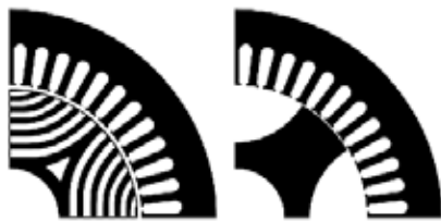
Fig. 1. General topology of a 4 pole SynRM with six flux barriers (left) and salient poles (right).
